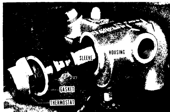
Fig. 17—Single Thermogard, Showing Element Removed from Housing
